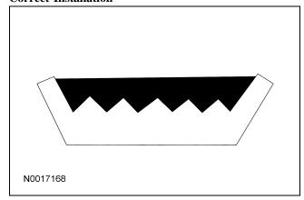
With the engine running, check accessory drive belt tracking on all pulleys. If the edge of the accessory drive belt rides beyond the edge of the pulleys, noise and premature wear will occur. Make sure the accessory drive belt rides correctly on the pulley. If an accessory drive belt tracking condition exists, proceed with the following:
