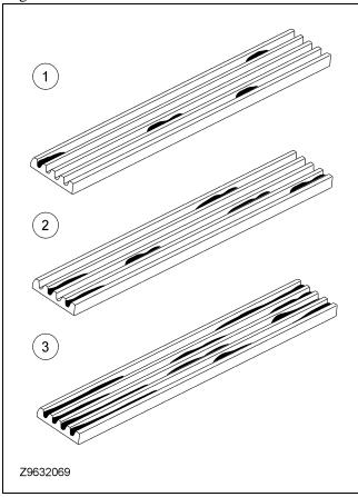
7. There should be no chunks missing from the belt ribs. If the belt shows any evidence of this, install a new accessory drive belt.
