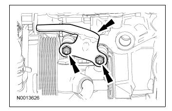
23. Remove the wiring harness retainer, nut and tube retaining clip from the power steering stud bolt.
