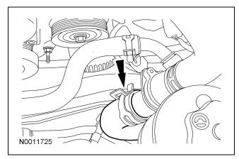
18. Disconnect the oil temperature sensor electrical connector and 2 pin-type retainers.
