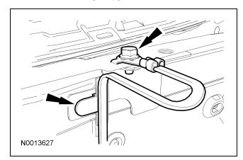
35. Disconnect the generator jumper harness electrical connector.
