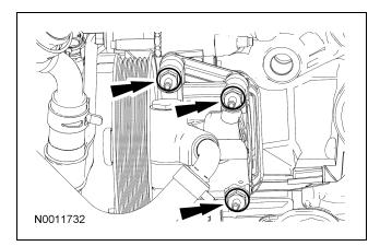
25. Install the special tool (lifting bracket) to the threaded hole located at the LH side of the engine block.
