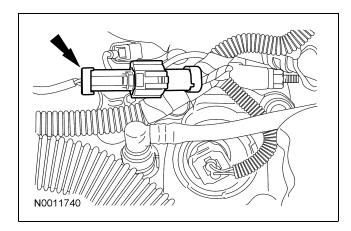
36. Disconnect the upper and lower powertrain control module (PCM) electrical connectors.
