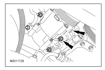
22. Remove the 2 nuts and the power steering pulley shield.
