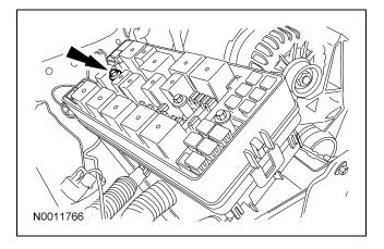
40. Remove the nut, radio interference capacitor and J-bracket from the engine front cover stud bolt.
