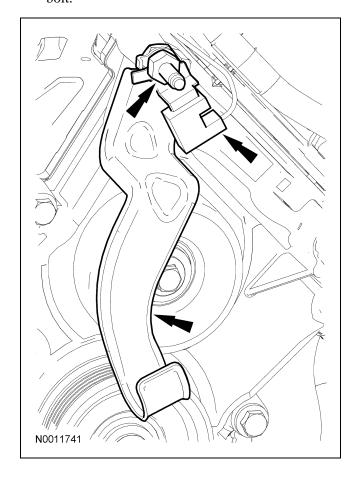
41. **NOTE:** RH shown, LH similar. Remove the RH and LH engine support insulator nuts.
