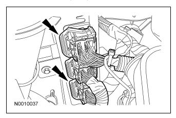
37. Disconnect the 16-pin electrical connector and detach the 2 wiring retainers.
