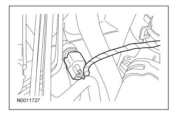
14. Disconnect the coolant hose from the oil filter adapter.
