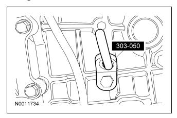
26. CAUTION: The rear of the engine must be supported before removing the transmission to prevent damage to the engine or cowl.
