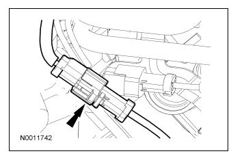
31. **NOTE:** RH shown, LH similar. Disconnect the RH and LH catalyst monitor sensor (CMS).
