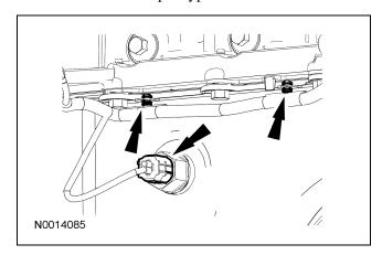
28. **NOTE:** Make sure the coolant hose is fully seated in the J-bracket.
