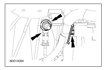
27. Connect the oil temperature sensor electrical connector and 2 pin-type retainers.
