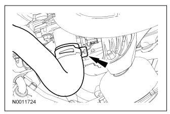
31. Connect the A/C pressure transducer electrical connector.
