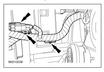
10. Connect the upper and lower powertrain control module (PCM) electrical connectors.
