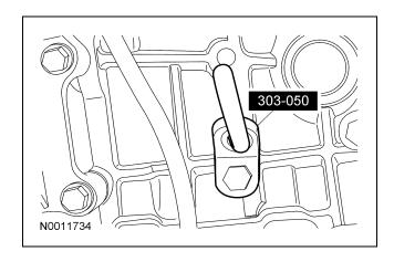
2. CAUTION: Do not remove the engine crane until the special tool (3-bar support) is installed in the next step. The rear of the engine must be supported to prevent damage to the engine or cowl panel.
