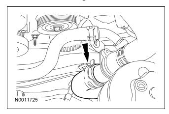
29. Attach the degas bottle hose to the cooling fan assembly.
