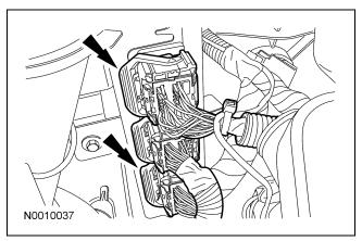
11. Connect the generator jumper harness electrical connector.
