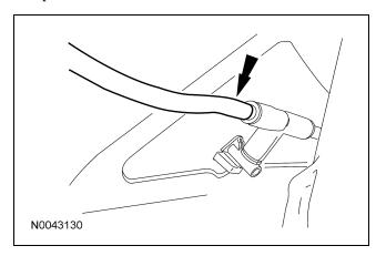
40. Install the hood insulation pin-type retainer and attach the 2 windshield washer hose retainers.
