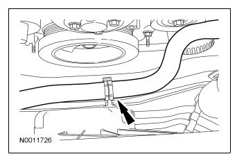
30. Connect the coolant hose to the oil filter adapter.
