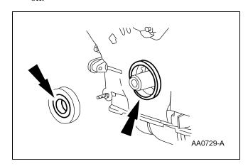
2. Using the special tools, install the crankshaft front seal.
