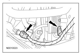
21. Detach the 2 wiring retainers from the FEAD bracket.
