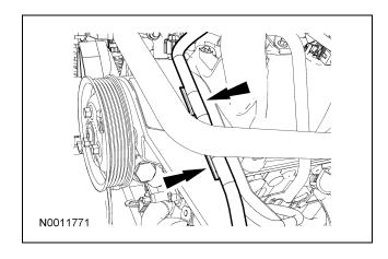
22. Disconnect the fuel supply tube coupling. For additional information, refer to Section 310-00.
