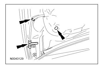
Position the hood insulation aside and disconnect the windshield washer hose.
