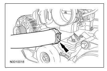
16. Disconnect the lower radiator hose from the coolant pump.
