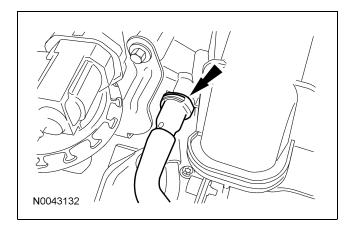
38. Disconnect the upper and lower powertrain control module (PCM) electrical connectors.
