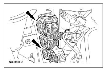
39. Disconnect the 16 pin electrical connector and detach the 2 wiring retainers.
