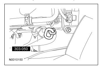
47. Install the special tool to the LH cylinder head.
