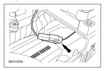
32. Disconnect the ignition coil electrical connector.
