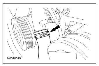
17. Remove the nut and power steering pressure tube bracket from the A/C compressor.
