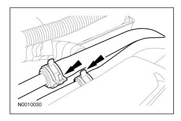
28. Remove the 2 coolant tube bracket bolts.
