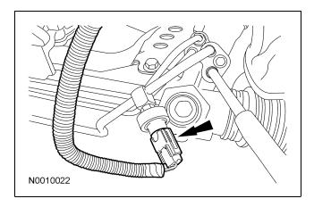
20. Disconnect the A/C compressor and A/C high pressure switch electrical connectors.
