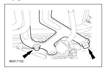
35. Detach the crankcase vent tube from the LH valve cover and remove the tube.
