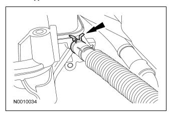
37. Disconnect the fuel vapor vent tube from the intake manifold.
