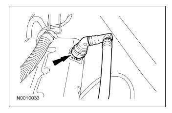
36. Disconnect the brake booster vacuum hose from the upper intake manifold.
