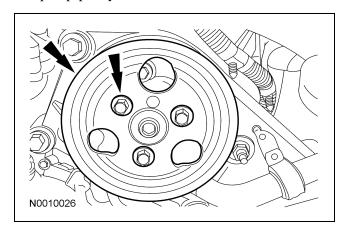
25. Remove the 3 bolts and position the power steering pump aside.
