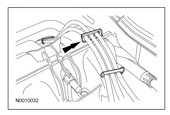
31. Disconnect the radio ignition interference capacitor electrical connector.
