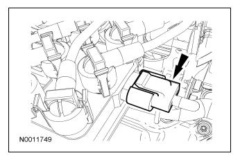
33. Remove the 2 upper ignition coil bracket bolts.
