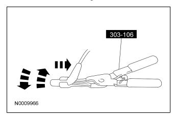
30. Detach the spark plug wire retainer from the intake manifold.
