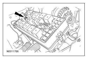
44. Remove the bolt and detach the ground cable from the RH strut tower.
