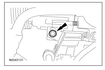
18. Remove the bolt and detach the power steering supply hose bracket from the front engine accessory drive (FEAD) bracket.
