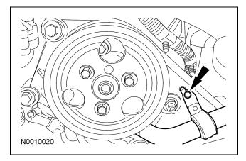
19. Disconnect the PSP switch electrical connector.
