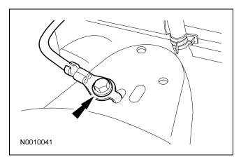
45. Detach the battery cable harness pin-type retainer from the cowl.
