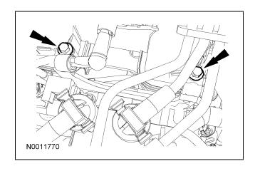
34. Remove the 2 lower ignition coil bracket bolts and then remove the ignition coil and spark plug wires.
