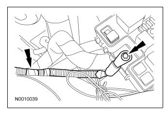
43. Detach the power distribution box upper housing from the lower housing, loosen the bolt and then disconnect the 68-pin connector from the power distribution box.
