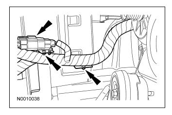
40. Detach the 3 wiring harness retainers.
