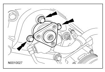
26. Remove the 3 bolts, the nut and position the FEAD bracket and A/C compressor aside.
