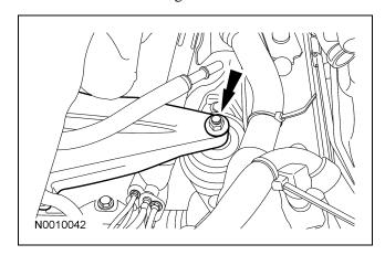
49. Remove the RH engine mount nut.
