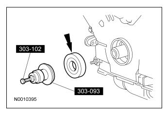
2. Install the crankshaft pulley. For additional information, refer to Crankshaft Pulley in this section.
