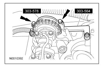
5. A CAUTION: The RH camshaft sprocket is a LH-threaded bolt.
