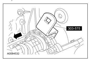
6. Remove the bolt and position the RH camshaft sprocket aside.
