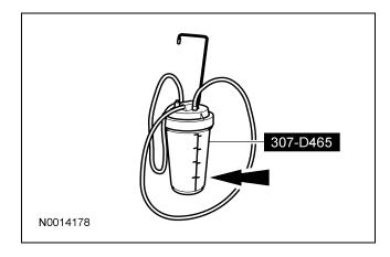
5. Hang the special tool under the vehicle, upright and close to the transmission.
