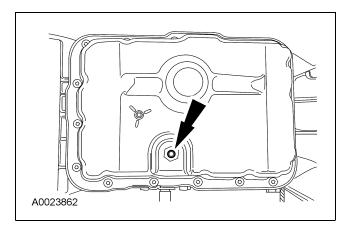
3. Install the special tool into the pan.
