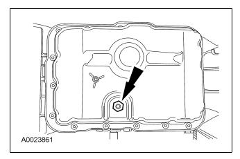
2. Hold the larger drain plug with a wrench and remove the small (center) fluid level indicating plug.
