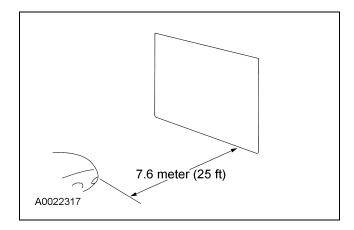
3. The correct visual aim for the fog lamps is with the top edge of the high-intensity zone 10 cm (4 in) below the horizontal center of the fog lamps.
