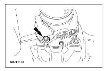
Using a suitable tool as shown, disconnect the driveshaft flanges from the flange pilots and remove the driveshaft.
