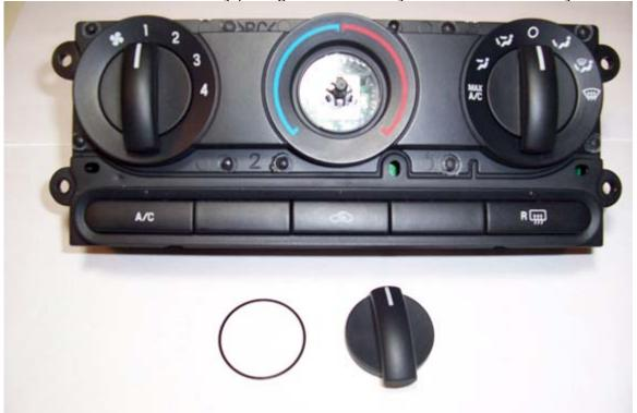
3. Depress the 4 tabs (2 each) on the top and bottom of the control module and separate the cover
