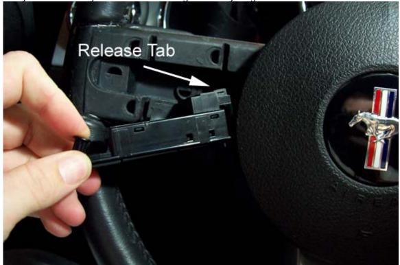
3. Once out there is one screw on the back and a few tabs securing the button assembly together.
