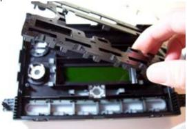
8. Remove the CD /AM-FM buttons by lifting the hinge-points and pushing them through the front of the face plate.
