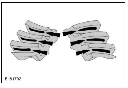
Correct backlash with a thicker pinion position shim required.
