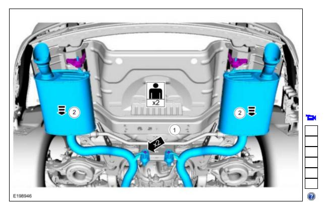
5. A WARNING: Align the new muffler and tailpipe component with the old muffler and tailpipe assembly to accurately mark the location to cut. Failure to cut the muffler and tailpipe in the correct location can result in an NVH concern or replacement of the entire muffler and tailpipe assembly.
