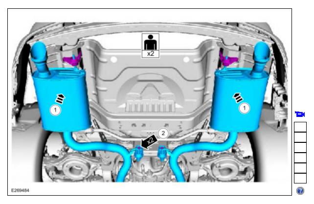
4. NOTE: Make sure the decorative tips are properly aligned with the openings in the rear bumper cover and adjust if needed.
