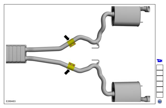
2. Tighten the clamps in the sequence shown. *Torque*: 35 lb.ft (48 Nm)
