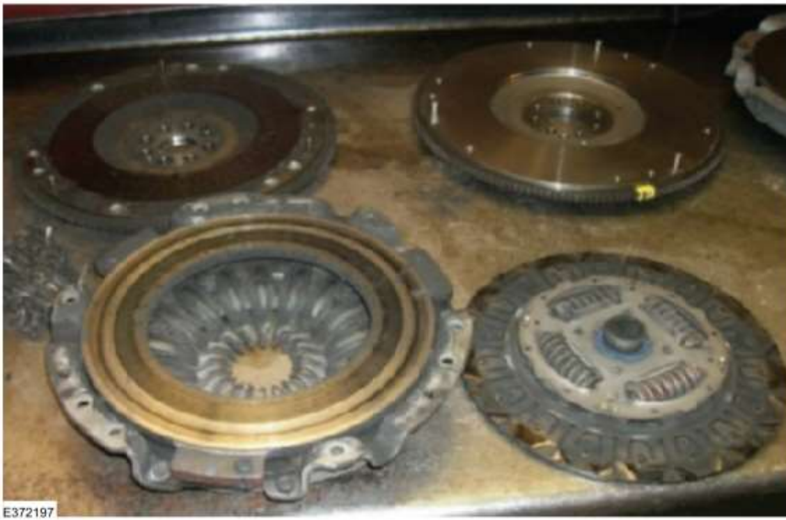
Clutch disc burst due to overspeed and excessive slip/heat. Figures show clutch lining material overheated, clutch binding agents burned off, clutch fibers loose in the clutch housing, jammed in pressure plate assembly. (Figure 6-7)
