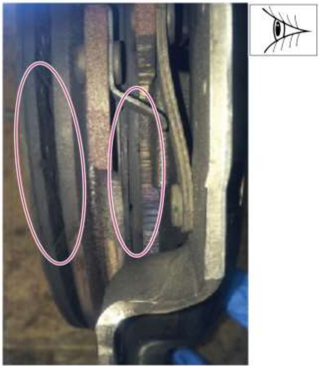
Reuse - Clutch flywheel showing normal heat-spotting marks that occur during break-in and normal use, with no adverse effect on function. (Figure 38-39)
