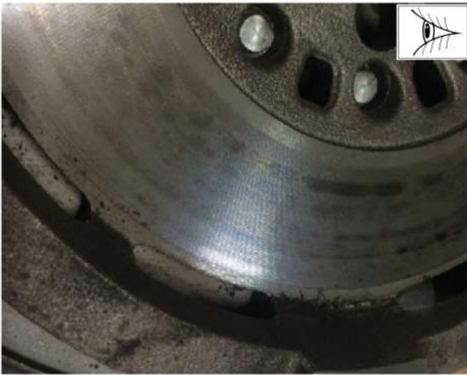
Not Reusable - Clutch flywheel showing material removed, blued, excessive lining dust. (Figure 40-42)
