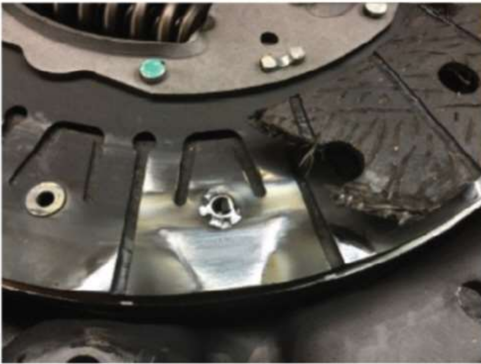
One side facing lost from each disc of a twin disc clutch due to overspeed / inadvertent downshift into 1st or 2nd gear at high vehicle speed. (Figures 3-4)
