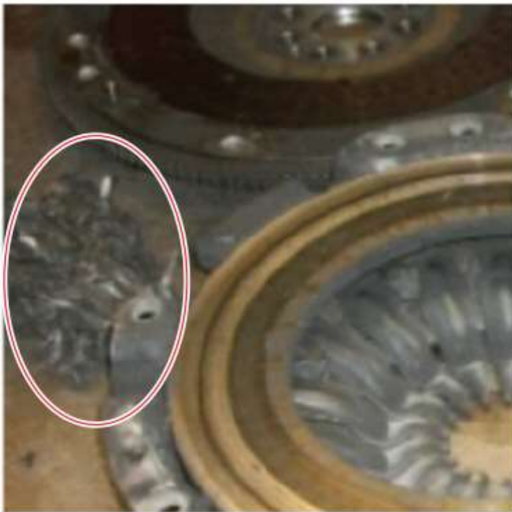
Clutch disc burst due to overspeed and excessive slip/heat. Figures show clutch lining material overheated, clutch binding agents burned off, clutch fibers loose in the clutch housing, jammed in pressure plate assembly. (Figure 6-7)
