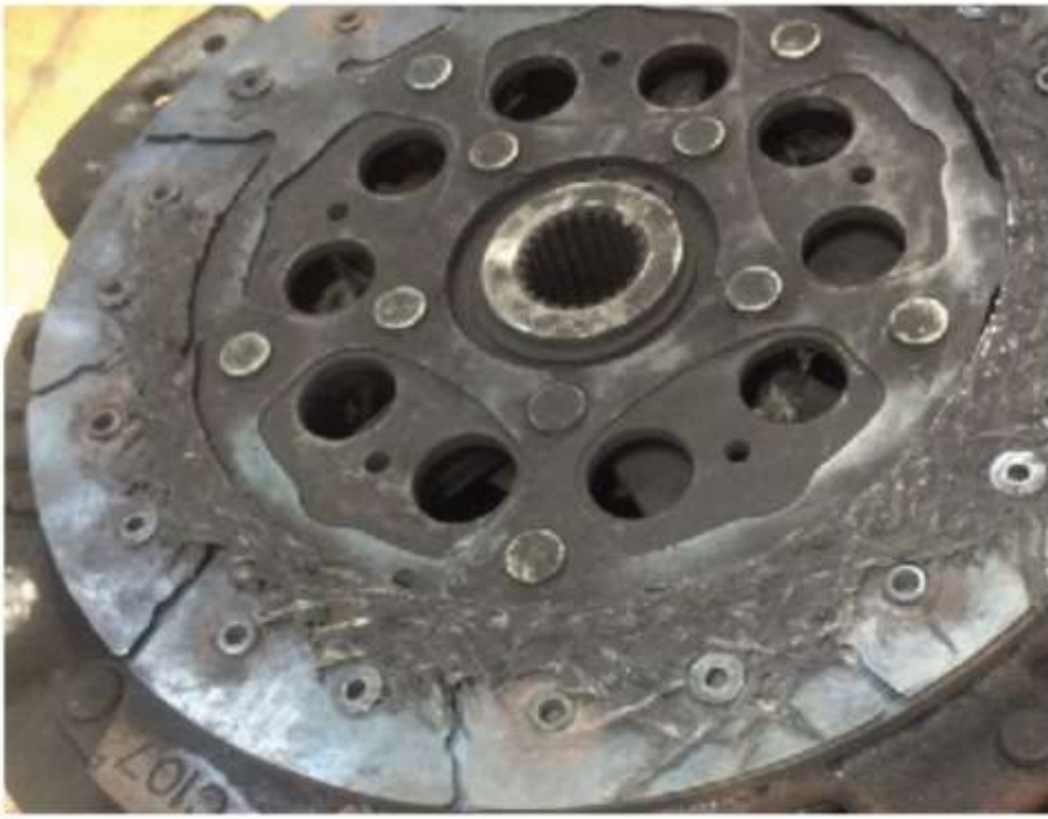
Clutch disc lining heat damage due to excessive slip. Figures show face and edge appearance of heat-damaged lining. (Figure 10-11)
