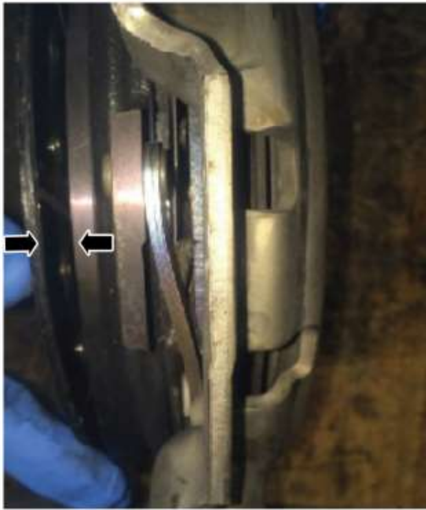
Clutch assembly is overheated due to excessive slip, with overspeed burst/'birds-nested' friction material fibers, overheated flywheel, overheated and scored pressure plate. (Figure 5)
