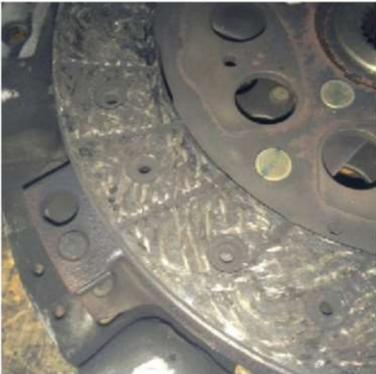
Clutch disc lining heat damage due to excessive slip. Figures show face and edge appearance of heat-damaged lining. (Figure 10-11)
