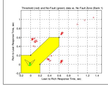
Example shown with lean-to-rich (0.2 sec), rich-to-lean (0.2 sec), and symmetric (0.6 sec) thresholds creating the yellow no-fault zone. The completeted monitor results in two measurements, a lean-to-rich response time and a rich-to-lean response time. These response time values are used as x-y pairs to make a single point and then compared to the no-fault zone. Anywhere in the yellow is a pass and outside the yellow is a failure.
