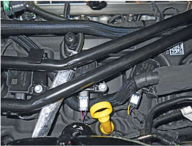
7. Connect the booster hose (1318-9D0692) to the supercharger and secure it with one (1) clamp (7329K11, found in 1318-TVSHWKD).
