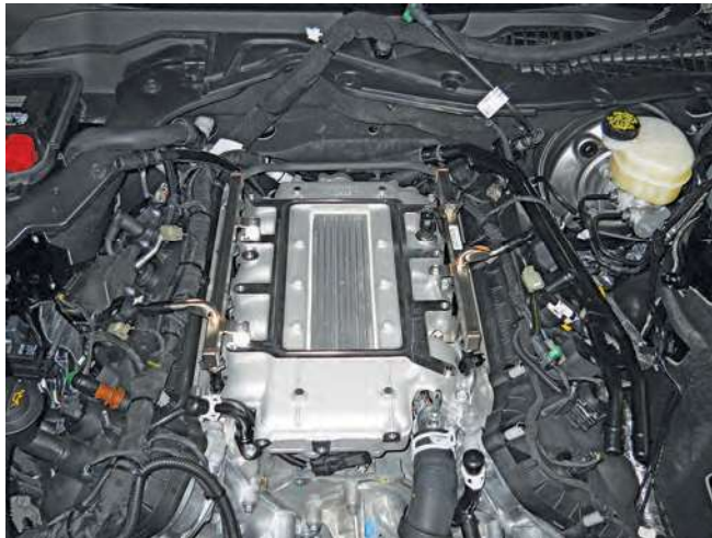
14. Connect the eight (8) fuel injector electrical connectors.
