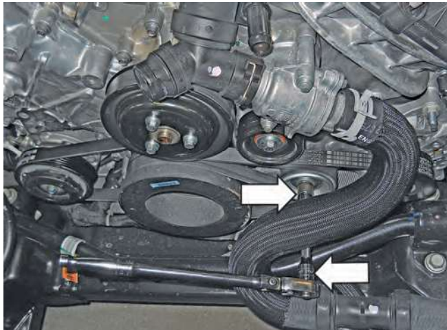
43. Cut and remove the A/C compressor belt. Discard the belt.
