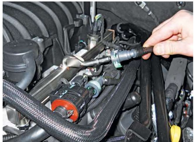
10. Install the fuel inlet line (green connector) to the tube on the LH fuel rail. Lock the connector.
