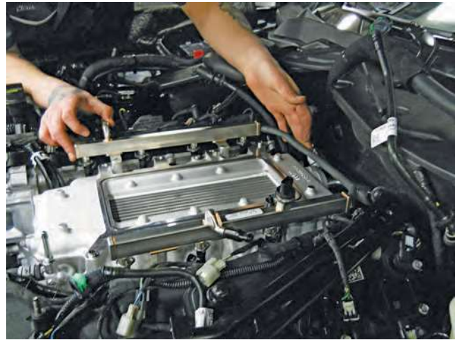
13. Install the M6x1.0x20 fuel rail-to-intake manifold bolt (BM6X20HF-S437) (short) at position 2 and M6x1.0x45 fuel rail-to-cylinder head bolt (161817) (long) at position 4. Tighten the bolts in two stages in the sequence shown. Stage 1: Torque the bolts to 10 Nm. Stage 2: Tighten the bolts an additional 45 degrees.
