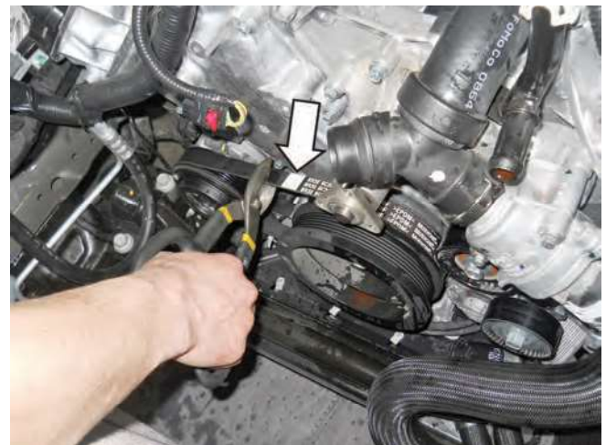
43. Cut and remove the A/C compressor belt. Discard the belt.
