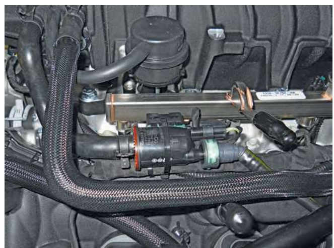
10. Install the fuel inlet line (green connector) to the tube on the LH fuel rail. Lock the connector.
