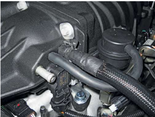
8. Install the hose (1318-9G272) between the supercharger and EECPV. Secure it with one (1) clamp (7329K11, found in 1318-TVSHWKD).
