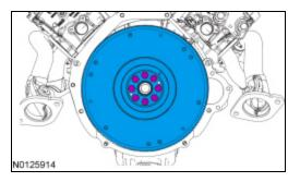
2. NOTICE: If installing a new pressure plate and/or flywheel, align the paint dot on the pressure plate as close as possible to the paint dot on the flywheel or a clutch system vibration can occur.
