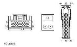
Are the resistances less than 3 ohms between the  $\underline{ACM}$  and the  $\underline{APIM}$ , and greater than 10,000 ohms between the  $\underline{ACM}$  and ground?
