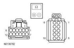
Are the resistances less than 3 ohms between the clockspring and steering wheel switches, and greater than 10,000 ohms between the clockspring and ground?
