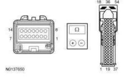
Are the resistances less than 3 ohms between the overhead console and the  $\underline{\text{APIM}}$ , and greater than 10,000 ohms between the overhead console and ground?
