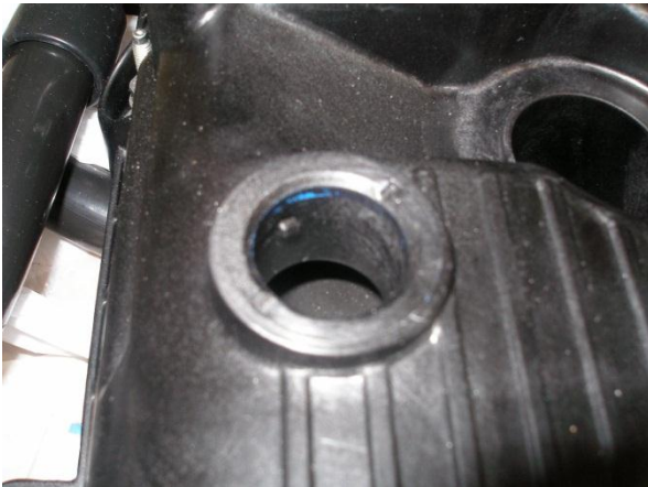
Rocker cover with nub for quarter-turn valve
