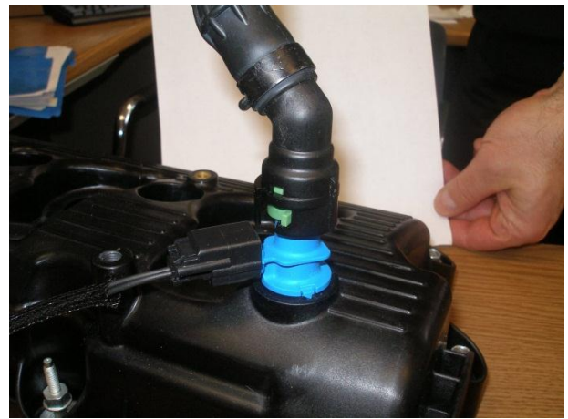
Assembled PCV system
