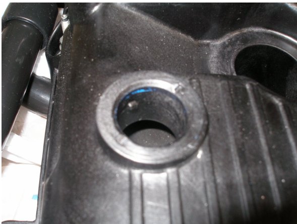
Rocker cover with nub for quarter-turn valve
