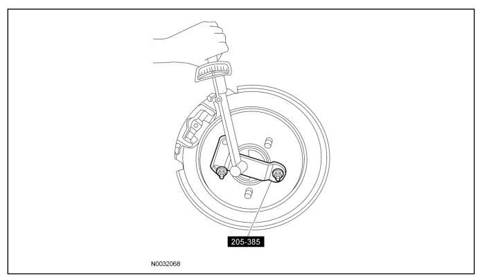
The axle shaft must turn with even pressure throughout the check without slipping or binding. If the torque reading is less than specified, check the differential case for incorrect assembly.
