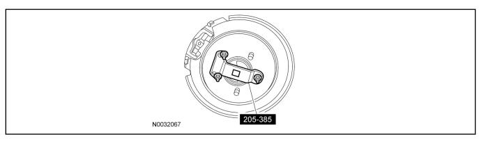
Use a torque wrench with the capacity of at least 271 Nm (200 lb-ft) to rotate the axle shaft. Make sure the transmission is in NEUTRAL, and that one rear wheel is on the floor while the other rear wheel is raised off the floor. The breakaway torque required to start rotation must be at least 27 Nm (20 lb-ft). The initial breakaway torque may be higher than the continuous turning torque.
