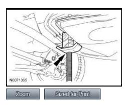
25. NOTE: Do not reuse the old transfer case-to-transmission bolts.
