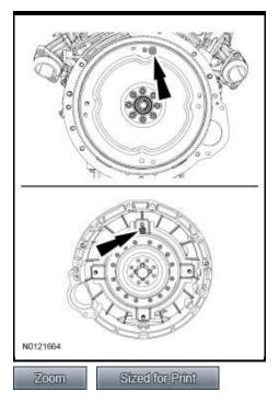
3. Install the Torque Converter Retainer.
