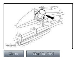
39. Separate the transmission fluid level indicator from the transmission fluid fill plug.
