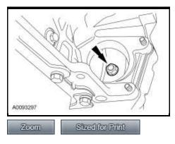
13. Install the rubber torque converter nut access cover.
