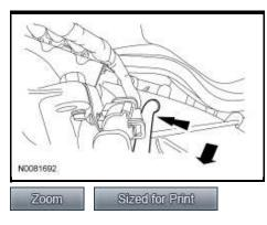
27. Connect the electrical connector and attach the 2 harness retainer clips to the transfer case.
