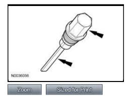
40. Wipe the transmission fluid level indicator clean. Reinstall the transmission fluid level indicator only back into the transmission fluid fill plug hole to check the transmission fluid level. Repeat this until a consistent reading is established.
