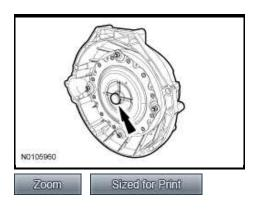
2. If equipped, align the torque converter stud and flexplate hole near the paint marks at the 12 o'clock position.
