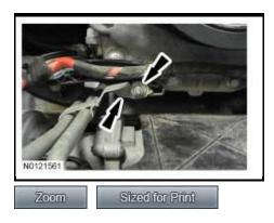
19. NOTE: Inspect the case to make sure the old transmission fluid cooler tube O-rings are not stuck in the case.
