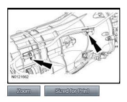
11. Connect the transmission electrical connector by pushing it in and twisting the outer shell to lock it in place.
