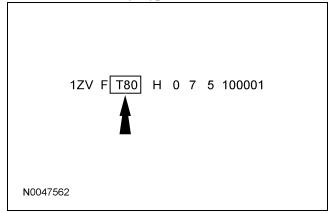
Positions 5 through 7 indicate vehicle line, series and body type.
