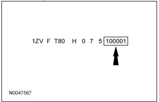
The last 6 VIN positions are the production sequence number. This number is also used as the vehicle serial and warranty number.
