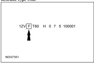
The fourth VIN position is the vehicle restraint system type code.
