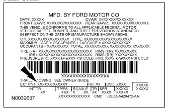
Paint codes may be listed as a 2-part code. The first set of paint code letters/numbers listed indicate the vehicle primary body color. The second set of paint code letters/numbers listed (if applicable) indicate a 2-tone or accent body color. All colors are base coat/clear coat.
