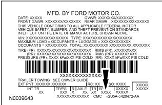
The spring code portion of the vehicle certification (VC) label identifies both the front and rear springs. The first set of characters listed indicate the front spring code. The second set of characters indicate the rear spring code.
