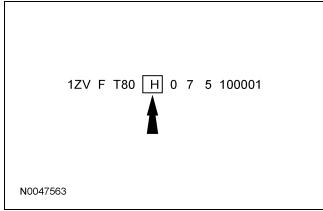
The eighth VIN position is the engine displacement and number of cylinders code.
