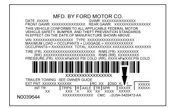
**NOTE:** Powertrain calibration information is limited to a maximum of 5 characters per line on the Vehicle Certification (VC) Label. Because of this, calibration identification consisting of more than 5 characters will wrap to the second line on the VC label.
