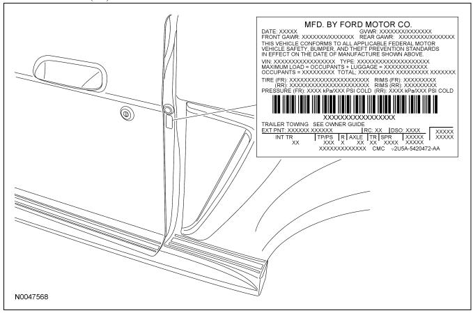
The upper portion of the vehicle certification (VC) label contains the manufacturer name, the month and year of manufacture, the certification statement and the vehicle identification number (VIN). It also includes gross vehicle weight ratings (GVWR). The VC label is located on the LH door jamb.
