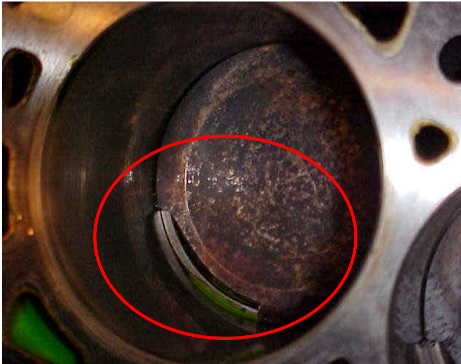
Upper Ring Land Broken
