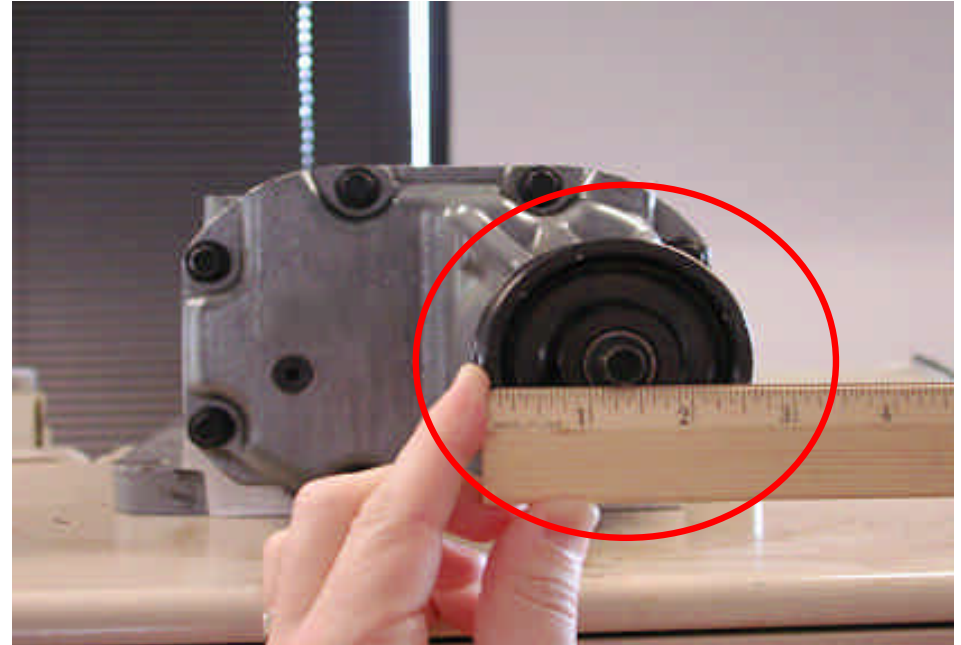
Modified (non-OEM) Supercharger Pulley
