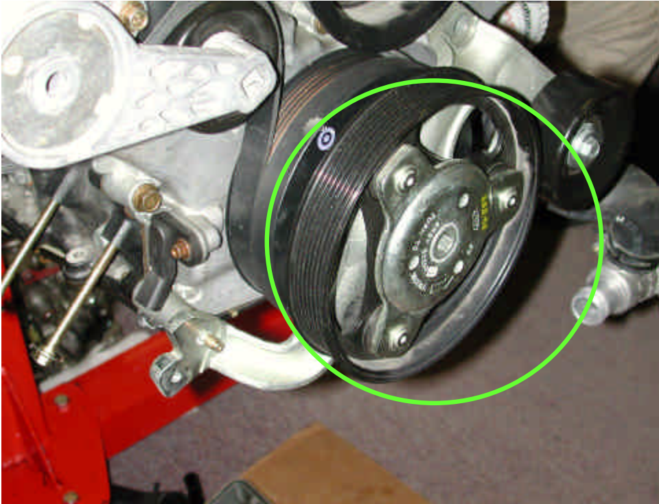
OEM Crankshaft Pulley for Supercharged Engines
