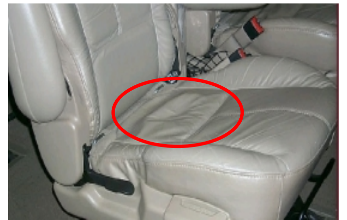
Baggy - excessive wrinkling
