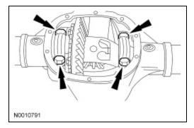
7. Rotate the differential assembly to make sure it rotates freely.
