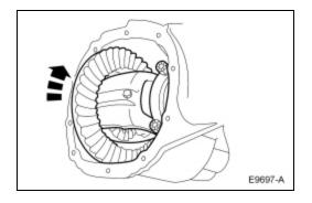
8. Adjust the ring gear backlash. For additional information, refer to Ring Gear Backlash Adjustment in this section.
