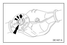
5. Using the Drive Pinion Flange Holding Fixture to hold the pinion flange, remove and discard the pinion nut.
