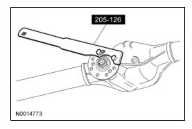
6. Index-mark the pinion flange in relation to the drive pinion stem to make sure of correct alignment during installation.
