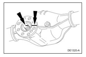
7. Using the 2 Jaw Puller, remove the pinion flange.
