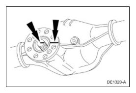
5. Using the Drive Pinion Flange Installer, install the pinion flange.
