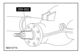
6. NOTICE: Install a new pinion nut with the same color as the original if not replacing the collapsible spacer. If a new collapsible spacer is installed, install the nut in the kit or damage to the component may occur.
