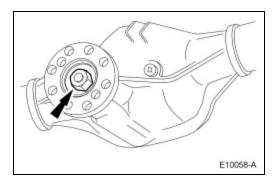
7. **NOTE:** Under no circumstances is the pinion nut to be backed off to reduce drive pinion bearing preload. If reduced drive pinion bearing preload is required, a new drive pinion collapsible spacer and pinion nut kit must be installed.
