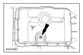
8. Install the special tool into the pan.
