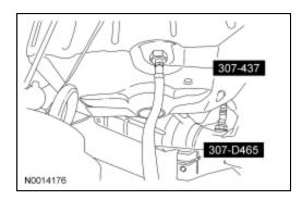
12. Apply a maximum of 206.85 kPa (30 psi) to the open end of the vacuum/pressure hose from the special tool. Fluid will immediately start flowing out of the special tool into the transmission fluid pan.
