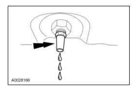
17. Reinstall the small (center) fluid level indicating plug and tighten to 10 Nm (89 lb-in).
