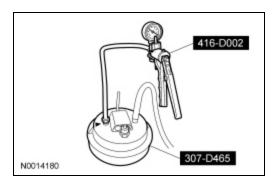
12. Allow the fluid to drain. When the fluid comes out as a thin stream or drip, the fluid is at the correct level.
