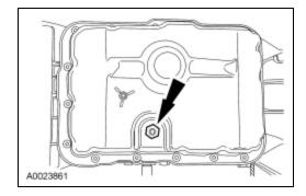
2. Hold the larger drain plug with a wrench and remove the small (center) fluid level indicating plug.
