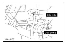
7. Apply a maximum of 206.85 kPa (30 psi) to the open end of the vacuum/pressure hose from the special tool. Fluid will immediately start flowing out of the special tool into the transmission fluid pan.
