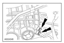
4. Turn on the pump and allow the transmission fluid to circulate a minimum of 5 minutes (cycling switch on and off will help dislodge contaminants in the cooler system).
