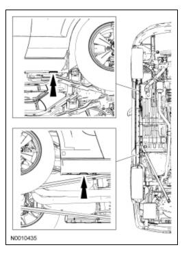
Lift the vehicle at the applicable lift points.
