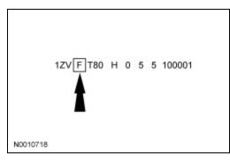
The 4th VIN position is the vehicle restraint system type code.
