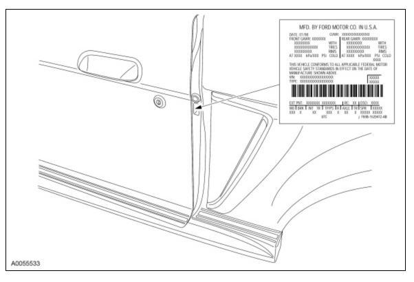
The upper portion of the vehicle certification (VC) label contains the manufacturer name, the month and year of manufacture, the certification statement and the VIN. It also includes gross vehicle weight ratings (GVWR). The VC label is located on the LH door jamb.
