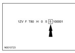
The 11th VIN position is the assembly plant code.
