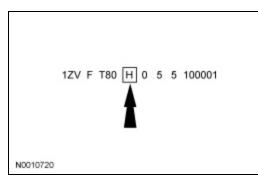
The 8th VIN position is the engine displacement and number of cylinders code.
