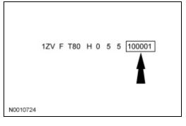
The last 6 VIN positions are the production sequence number. This number is also used as the vehicle serial and warranty number.
