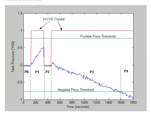
P0 = Phase 0, Stabilization Phase – With CVS open, Tank Pressure is allowed to stabilize. A fuel volatility test is performed and FTPT offset correction is learned if volatility test passes.
