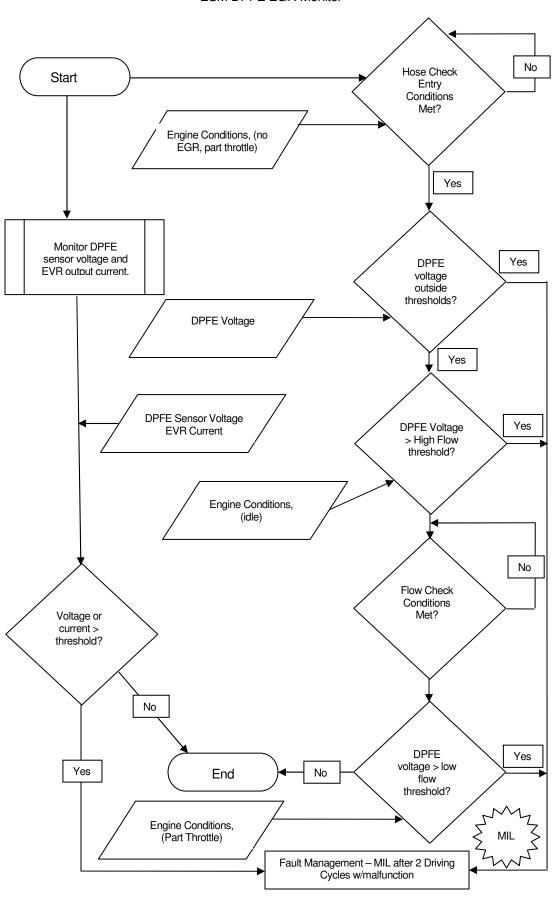
The ESM Delta Pressure Feedback EGR Monitor is a series of electrical tests and functional tests that monitor various aspects of EGR system operation.
