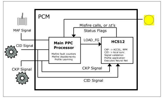
"Profile correction" software is also used on NNM systems to "learn" and correct for mechanical inaccuracies in crankshaft tooth spacing under de-fueled engine conditions (requires up to three 60 to 40 mph no-braking decels after Keep Alive Memory has been reset). These learned corrections improve the high rpm capability of the monitor. The misfire monitor is not active until a profile has been learned.
