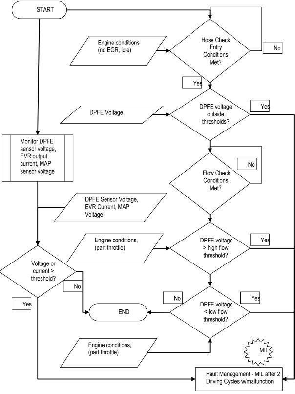
The ESM Delta Pressure Feedback EGR Monitor is a series of electrical tests and functional tests that monitor various aspects of EGR system operation.
