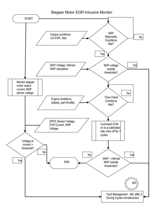
The Stepper Motor EGR Monitor consists of an electrical and functional test that checks the stepper motor and the EGR system for proper flow.
