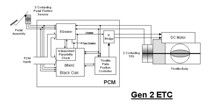
Because safety is a major concern with ETC systems, a complex safety monitor strategy (hardware and software) was developed. The monitor system is distributed across two processors: the main powertrain control processor and a monitoring processor called an Enhanced-Quizzer (E-Quizzer) processor.
