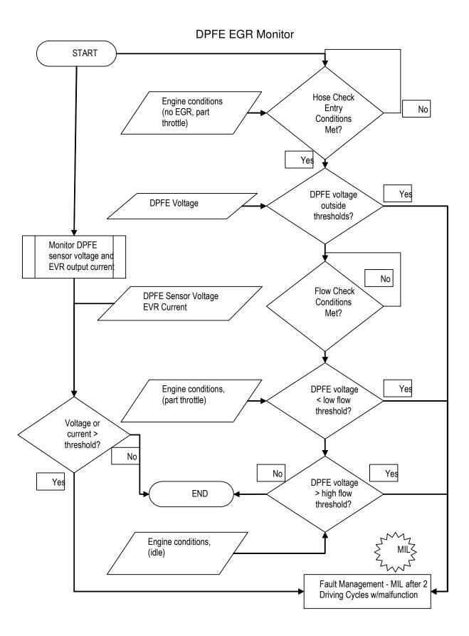
The Delta Pressure Feedback EGR Monitor is a series of electrical tests and functional tests that monitor various aspects of EGR system operation.
