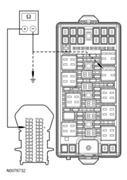
Is the resistance less than 5 ohms between the SJB and the BEC, and greater than 10,000 ohms between the SJB and ground?
