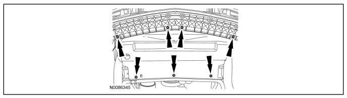
3. Remove the 6 pushpin retainers and the air deflector.
