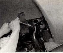
At the former quad shock mounting **B**location, the bolt threads right into the bracket that has an adjustable nut inside.
