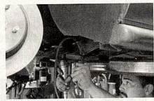
The front of the IRS cradle simply 9 attached directly to where the lower control arms used to go. Once the bolt is all the way through on each side, the nut can be attached and the entire piece tightened up. At this point, the biggest step, actually installing independent rear suspension in an SN-95 Mustang that didn't originally have it, is finished.
