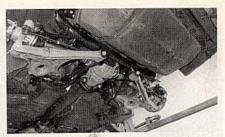
The installed IRS in the Currie '95 GT looks like this. Another nice incidental is that the existing driveshaft works fine with the IRS. Making it longer or shorter is a hassle you don't have to deal with. It's also a great time to upgrade to an FRPP aluminum driveshaft as will soon be done with this car.
