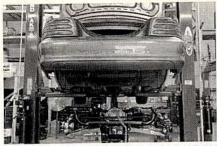
It's interesting to note that most of the Obrain power for installing the IRS was used to come up with a good way to secure the mounting brackets to the car. Once those were on and bolted down, installing the entire IRS assembly was only a matter of raising the assembly up into the car and securing it to the four existing pickup points with nuts, washers, and bolts. Here, we were ready for that next dramatic step.
