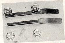
The finished piece above is ready for Zits permanent placement inside the car's framerail. The nuts are spaced about 3% inches apart, and Currie bent the piece of bar stock on the end to create the handle as shown.
