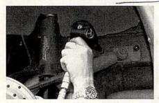
The quad shocks come off and go by the 5 The quad snocks come on and steem in wayside. The bracket that holds them in place on the car needs to be removed as well, so it's easier to remove the entire assembly at the same time—shocks, brackets, and all.
