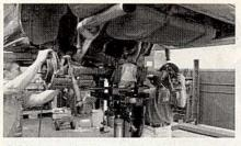
**6**Disconnecting the upper and lower control arms at the car and leaving them attached to the rearend is the easiest way to get the entire assembly off at once. Once those are unbolted, the entire rearend drops out of the car upon disconnection of the brake lines, shocks, and driveshaft. Once the rearend is out of the car, unbolting and removing the exhaust pipes is simply a matter of removing them from the mufflers and disconnecting them from their hangers.
