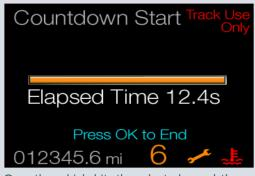
Once the vehicle hits the selected speed, the screen instantly displays the elapsed time.
