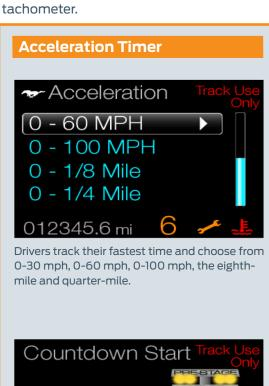
Both an automatic start and a countdown start, with a drag racing start light, are available.
