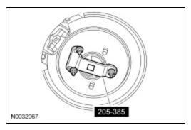
Use a torque wrench with the capacity of at least 271 Nm (200 lb-ft) to rotate the axle shaft. Make sure the transmission is in NEUTRAL, and that one rear wheel is on the floor while the other rear wheel is raised off the floor. The breakaway torque required to start rotation must be at least 27 Nm (20 lb-ft). The initial breakaway torque may be higher than the continuous turning torque.
