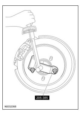
The axle shaft must turn with even pressure throughout the check without slipping or binding. If the torque reading is less than specified, check the differential case for incorrect assembly.
