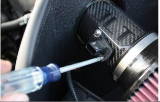
Plug in the MAF, PCV and automatic line (if used). Adjust tube for best fit and lightly snug all clamps.
