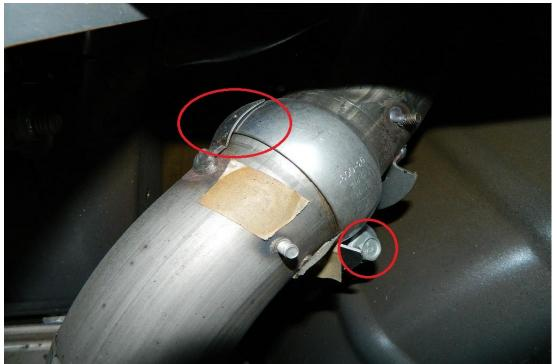
2. Remove rubber holder from muffler. This takes some effort. I used my body to help support the muffler while doing this.
