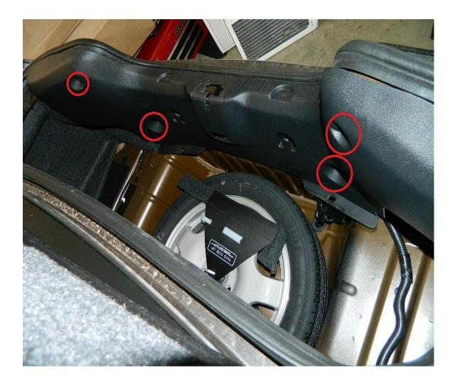
2. Unscrew (3) screws from rear splash guard and then unclip rear splash guard and remove. (Both sides). This is made much easier by removing the rear wheels, I used a ¼ hex head on a wrench with a phillips head bit on the end to get them out. Not ideal, but it worked.
