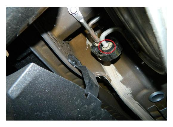
3. Once free, push up on mid pipe and separate ball joint of muffler from pipe. This also takes some effort. (Picture shows bolt still tightened, yours will be loose at this point.)
