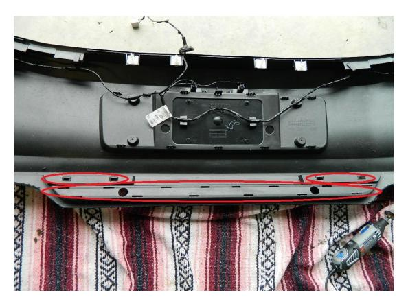
2. Along the inside, Ford drew a line for where to cut the bumper, as well as (9) slits for the new valance to clip into. Because of the angle of the Dremel, I drilled holes along the line every few inches and did a decent portion of the Dremel cutting from the outside of the bumper. Not ideal, but it worked. A body saw would prevent the need for this.
