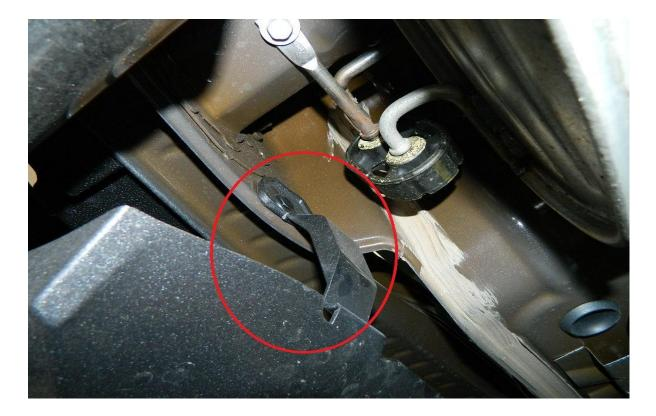
5. Once bumper is snapped on, reinstall push pins on plastic arms and included white plastic locks. Reinstall push pins under side of bumper next to mufflers, and then the rear splash guard and its screws. Reinstall taillights, and then the inner trunk plastic panel.
