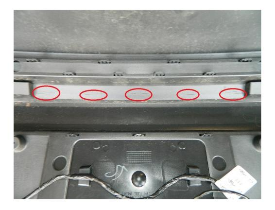
3. New valance snaps into place. Make sure to check that it is fitting correctly and make additional cuts/adjustments as needed. Snap in red reflectors.
