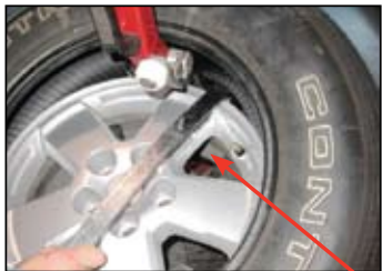
Bottom Bead Removal (Critical step)
