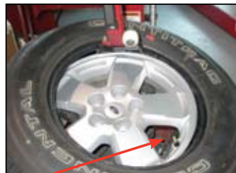
Top Bead Installation
