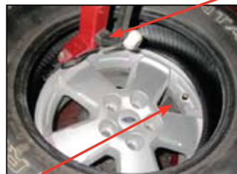
Bottom Bead Installation
