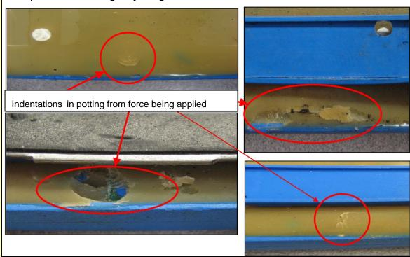
Example of Sensor Torn Off Cradle By Tire Machine
