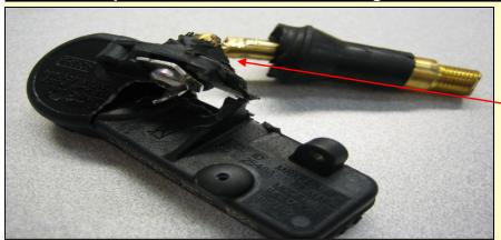
Severe chassis damage from attempting to pull the valve out with sensor attached
