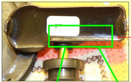
Detail of housing showing potting separation due to heavy force applied to the valve. If a finger nail or business card can be inserted between the TPMS sensor housing and potting, the TPMS sensor has been damaged. Damage of this nature is most often caused by improper tire removal or attempting to remove the valve stem like a conventional rubber valve stem.
