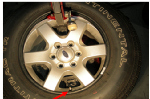
Bottom Bead Installation
