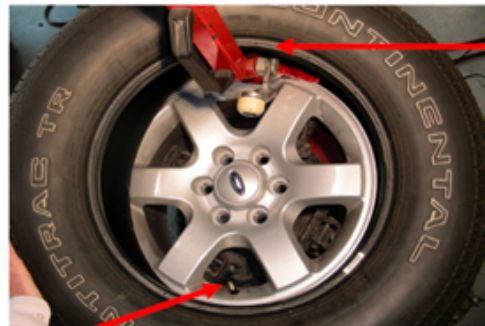
Top Bead Installation
