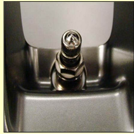
Bolt-On Stem Note: Nickel Plated Brass Valve Sensor Type 7
