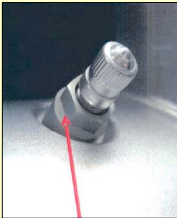
Bolt-On Stem Note: Aluminum Nut Sensor Type 1&2
