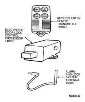
The electronic door lock control processor performs the following functions:
